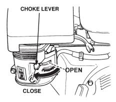
Figure 11. Choke Lever
